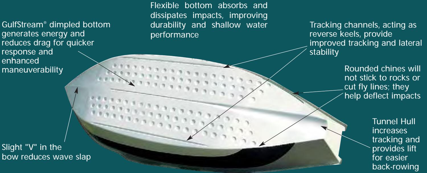
Designed to work in harmony with the Tunnel Hull®, the Gulfstream® dimpled bottom reduces drag in moving water and has received outstanding reviews from guides and outfitters throughout North America. Here at ClackaCraft, we feel the dimples are so effective that we have engineered them into all of our hulls 15' and larger. Our boats simply row better. Try one, we think you'll agree.
